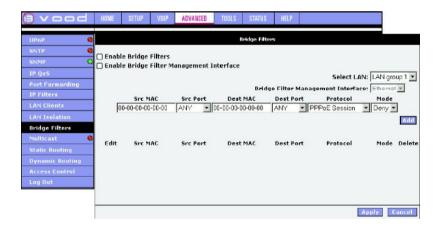
When bridge filtering is enabled, each frame is examined against each defined filter rule sequentially, and when a match is found, the appropriate filtering action (determined by the access type selected ... i.e. allow or deny) is performed. The user should note that the bridge filter will only examine frames from interfaces that are part of the bridge itself. Up to twenty filter rules are supported with bridge filtering.
