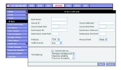
This page is invoked when you click on the **Add** button of "**QoS Setup Page**". This page allows you add a rule or matching criteria that identifies an application traffic. The application traffic can be identified by rule name, source/destination IP address and netmask, source/destination port range, protocol and traffic priority.
