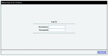
Use the default user name **Conf** and password **admin** for first time setup. You should change the web-based manager access user name and password after you have verified that a connection can be established. The user name and password allows any PC within the same subnet as the Vood unit to access the web-based manager.
