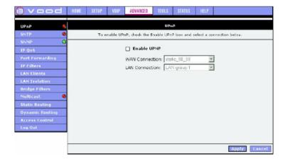
UPnP NAT and Firewall Traversal allow traffic to pass-through the router for applications using the UPnP protocol. This feature requires one active connection. In presence of multiple connections, select the one over which the incoming traffic will be present, for example the default Internet connection.
